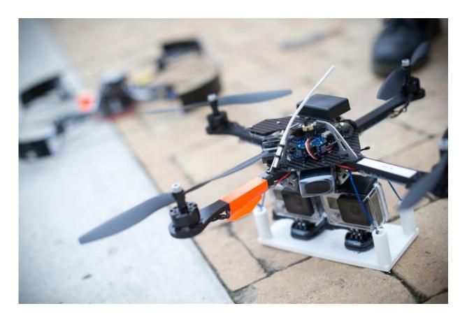
An Ascending Techologies Hummingbird quadcopter, which serves as the base UAV for wireless recharging of sensors, monitoring of crops and measuring of water. Credit: Randall Gee, University of the Pacific, CC BY-ND
