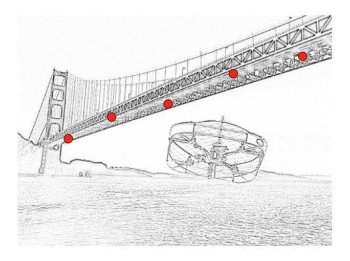
Idealized figure representing a number of sensors (in red) monitoring a bridge and the UAV flying to wirelessly recharge the sensors' batteries. Credit: Carrick Detweiler, University of Nebraska-Lincoln, CC BY-ND
