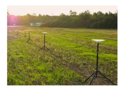
Bioaerosols deposition sampler array set up at the edge, and downwind, of a manure-applied field. Credit: Shane Rogers.
