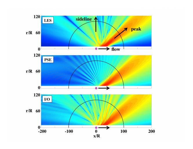
Contours of decibel levels of the sound emitted from a supersonic jet. The nozzle exit is located at the magenta dot in each figure, and the jet flows from the nozzle to the right. Jet noise is computed using high-fidelity large eddy simulation (LES) in the top panel, using one wavepacket computed from the parabolized stability equations (PSE) in the middle panel, and through a superposition of input-output (I/O) modes from the new analysis technique in the
