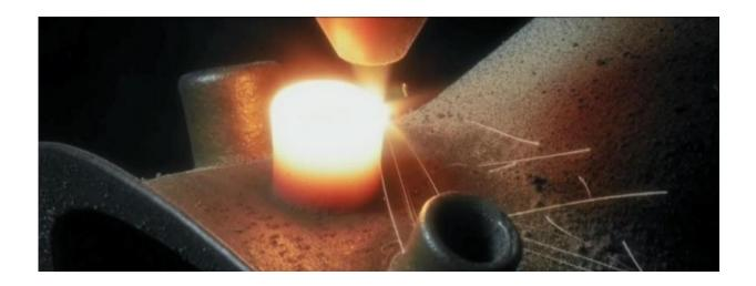
In additive manufacturing, also known as 3D printing, components are built up layer by layer – in other words as an additive process – on the basis of threedimensional design data. Siemens Corporate Technology (CT) is contributing its expertise primarily to the development of materials and the simulation of the production process. Laser melting is the most important method used by Siemens in the area of additive manufacturing.
