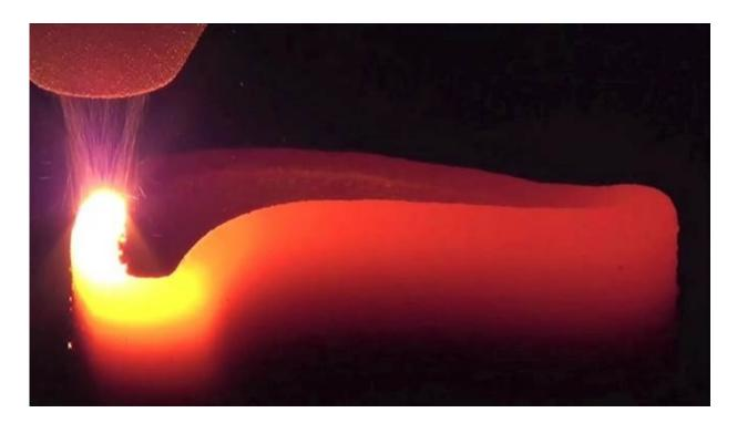
Lasers are increasingly being used in places where objects were previously forged, milled or cast. Laser beam welding creates objects layer by layer.
