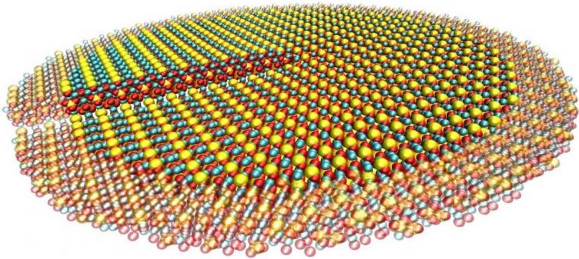
A computer model shows tricalcium silicate with a defect known as a screw dislocation, which influences the brittle properties of the crystal structure. The atoms on the periphery are faded because they are little affected by the dislocation core at the center of the disc. Credit: Lei Tao
