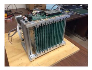
Missouri S&T researchers have produced a 3-D microwave video camera that is small and portable, making it easy to use in many applications.
