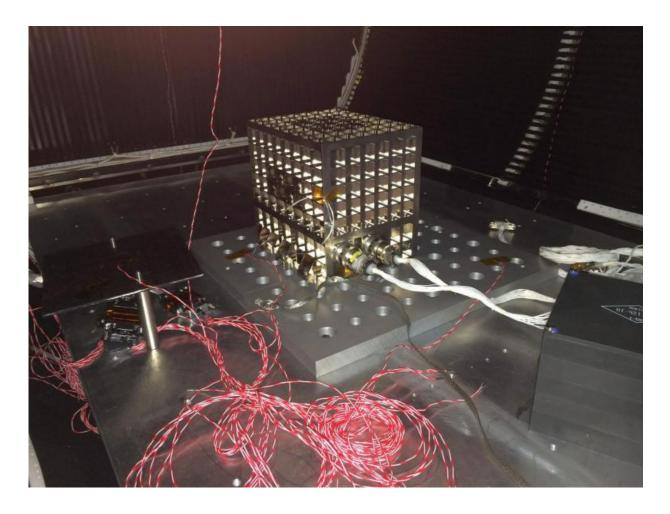
Crude oil experiment thermal-vacuum testing. Credit: ESA-A. Verga
