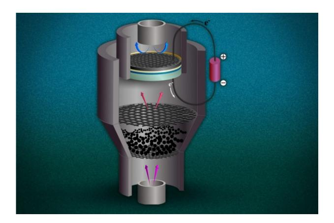
This illustration depicts a possible configuration for the combined system proposed by MIT researchers. At the bottom, steam (pink arrows) passes through pulverized coal, releasing gaseous fuel (red arrows) made up of hydrogen and carbon monoxide. This fuel goes into a solid oxide fuel cell (disks near top), where it reacts with oxygen from the air (blue arrows) to produce electricity (loop at right). Credit: Jeffrey Hanna
