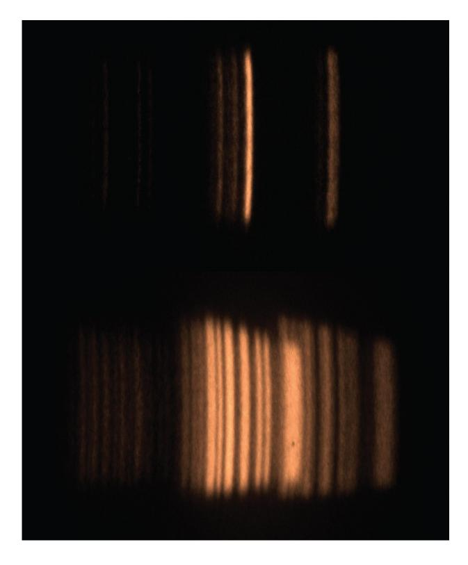
The top image shows a typical reading from a mass spectrometer, where each line indicates the presence of a certain substance. The bottom image shows a reading from the new coded aperture, where researchers rely on computers to
