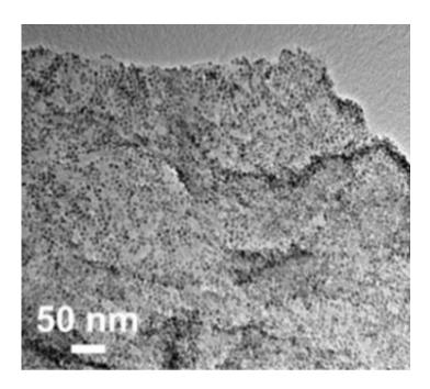
Nitrogen-rich graphene festooned with finely tuned copper nanoparticles selectively converts carbon dioxide to ethylene, a key commodity chemical. Credit: Sun Lab / Brown University
