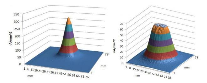
The difference in beam distribution on the target with the raster system off (left) and with the raster system on (right). The different color bands delineate the y-scale divisions, which are different on each plot. Note that although the total integrated beam density is equivalent in both plots, the peak beam density is five times higher when the raster system is off. The raster system clearly provides a more even beam distribution on the entire target.
