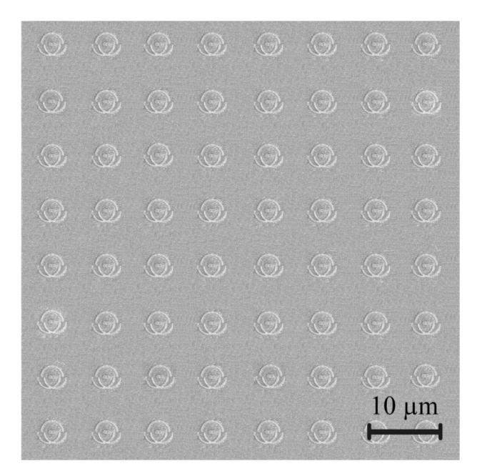
The nanophotonic chip designed by Australian researchers, magnified 2000 times. Each indentation on the image is a single unit of the chip -- like a single pixel in a display panel -- made up of semi-circle nano-grooves and nanoapertures engraved in a metallic film. These single units can be individually controlled to manipulate the angular momentum of light (AM) at a chip scale. Credit: RMIT University
