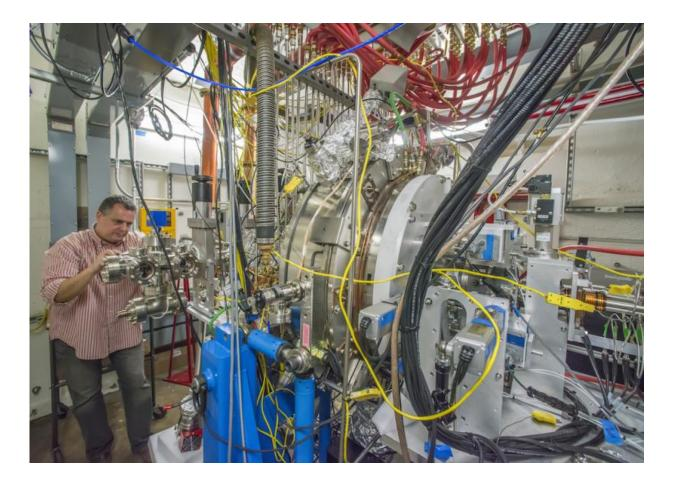
Berkeley Lab's Fernando Sannibale inspects the APEX (Advanced Photoinjector Experiment) that has served as a test electron gun and injector system for LCLS-II. The LCLS-II injector system will be located at the future X-ray laser's front end. It will produce bunches of electrons for the generation of X-ray pulses that are only quadrillionths of a second long, at rates of up to a million bunches per second. Credit: Roy Kaltschmidt/Berkeley Lab
