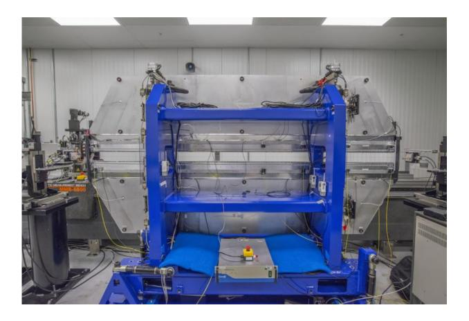
A prototype LCLS-II undulator, which is designed to wiggle electrons, causing them to emit brilliant X-ray light, undergoes magnetic measurements at Berkeley Lab. Credit: Roy Kaltschmidt/Berkeley Lab
