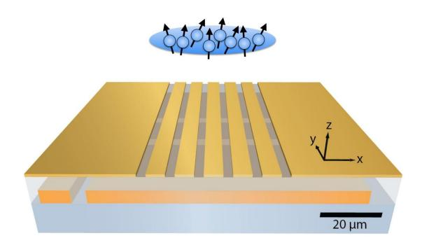
A microchip is used to trap a cloud of ultracold atoms and to entangle the atoms' magnetic moments. Credit: University of Basel, Department of Physics
