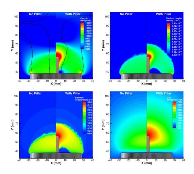
In research at Purdue, a simulation technique may help to reduce the cost of carbon nanostructures for research and commercial technologies, including advanced sensors and batteries. These graphs show how including a "dielectric
