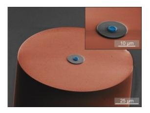
Researchers used femtosecond laser writing to fabricate an optical element known as a phase mask (blue) onto a base (gray) that sits directly on the center of an optical fiber. This electron microscopy image has been colorized. Credit: Timo Gissibl, University of Stuttgart
