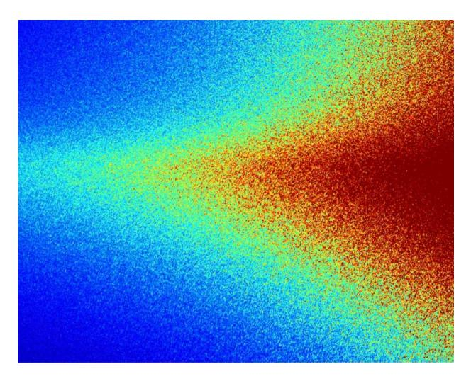
A beam of X-rays scattering off a thin film of silicon form this speckle pattern that corresponds to the details of the surface. University of Vermont scientists used these kinds of images as part of a discovery that is providing a new view at the nanoscale. Credit: Randall Headrick, UVM
