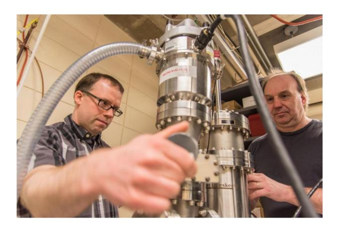
University of Vermont physicists Jeff Ulbrandt and Randy Headrick have discovered a novel way to mix X-rays -- opening a new window onto atoms in motion. Using this vacuum chamber, they created thin films like those used in solar panels and LCD screens -- while shining X-rays on them at the Argonne National Laboratory. Within their gigabytes of data, the scientists found an unprecedented view of the messy motion of complex objects at the nanoscale. Credit: Joshua Brown, UVM
