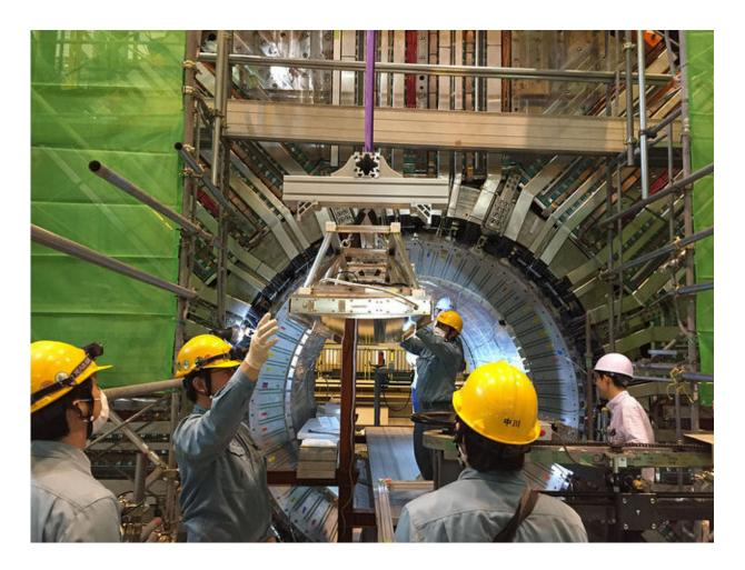
Scientists and technicians insert one of the optical components of the iTOP detector into the Belle II detector in February 2016.
