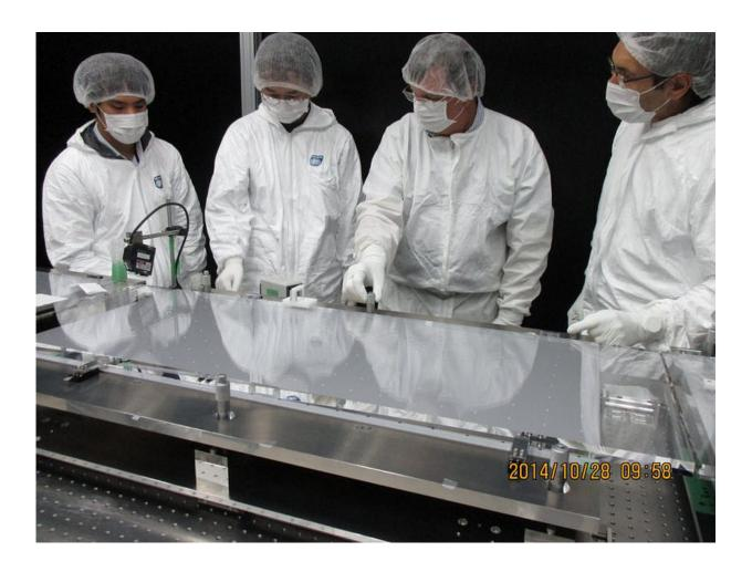
PNNL scientist James Fast (second from right) and colleagues check one of the 16 quartz components or "planks" of the imaging Time of Propagation detector.
