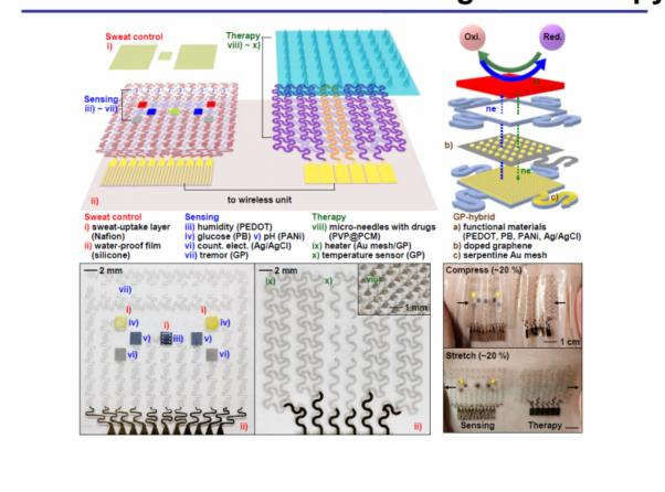
Figure 1. Schematic and corresponding images of the GP-hybrid electrochemical devices and thermoresponsive drug delivery microneedles. Credit: IBS
