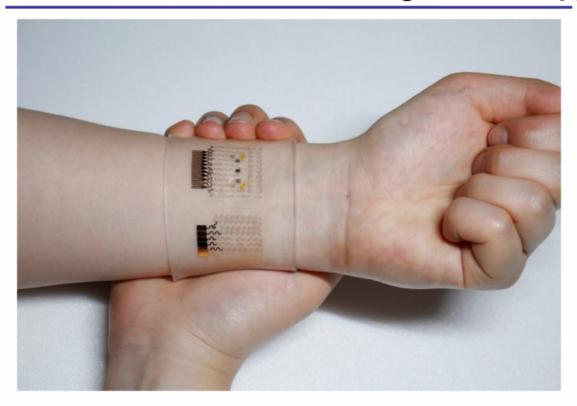
Figure 2. Optical image of the GP-hybrid electrochemical device array on the human skin Credit: IBS
