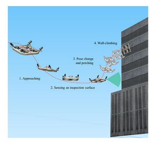
Concept of CAROS, a drone-type wall-climbing robot system. Credit: KAIST
