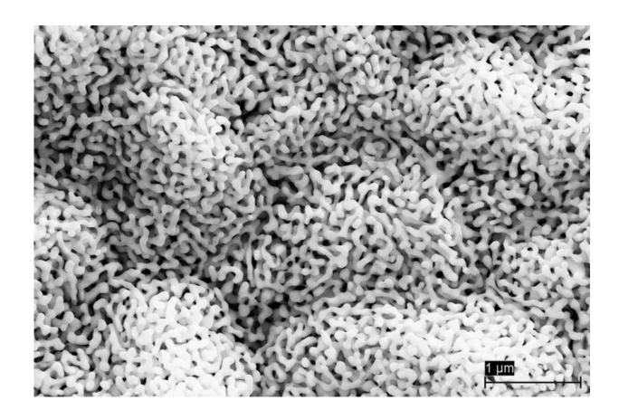
In order to be able to control each point of light independently a gold nanosponge establishes the contact between each individual pixels and the driver chip. The nanoporous gold structure compresses like a real sponge and can be precisely adapted to the topography of the component. Credit: Fraunhofer IZM
