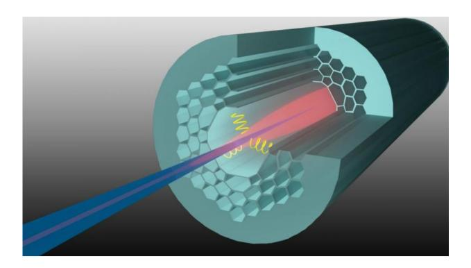
Simple, self-aligning method traps tiny tapered glass fiber inside hollow-core optical fiber, with potential applications in laser cutting and basic physics research. Credit: Philip Russell, director at the Max Planck Institute for the Science of Light in Erlangen, Germany
