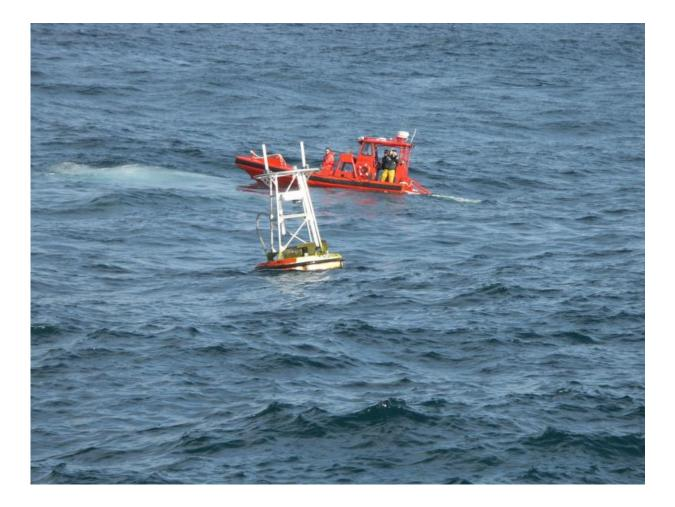
Breaking away: NOAA tsunami detection buoys can come unmoored in the deep ocean, as this one did, requiring recovery and replacement – and not detecting any usable data until it's back in place. Credit: LCDR Mark Wetzler, NOAA
