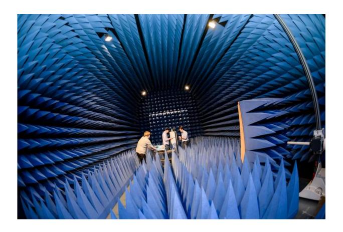
The development of a new device for the detection of land mines begins with tests in a highly controlled environment, for example in this chamber which absorbs electromagnetic waves. Credit: RUB, Damian Gorczany
