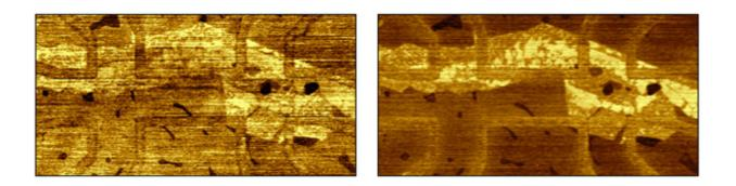
Local surface potential maps for synthetic air (left) and ambient air (right), with the same relative humidity of 40%. The scan size is  $6\times3$  micrometres squared.
