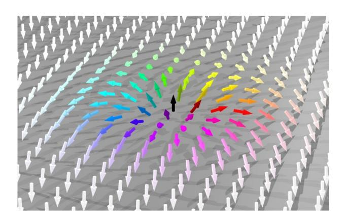
The magnetic structure of a skyrmion is symmetrical around its core; arrows indicate the direction of spin. Credit: ill./©: Benjamin Krüger, JGU
