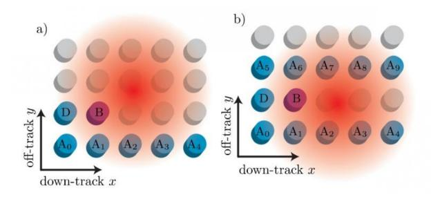
Illustration of two versions of the HAMR writing procedure, showing a laser being used to heat bit B, which enables the bit to be written by a much smaller magnetic field than would otherwise be required. All of the surrounding A bits remain in their original states because they have not been heated (enough), and so cannot be written by the magnetic field. Credit: Vogler, et al. ©2016 AIP Publishing
