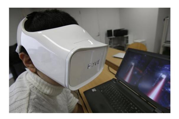
In this March 7, 2016 photo, Fove's staff wearing an eye-tracking headset goggles demonstrates virtual reality at his office in Tokyo. San Francisco-based startup Fove has developed eye-tracking for virtual reality - that kernel of technology many feel is key for the illusion of becoming immersed in a setting. Fove has devised a way to use tiny infrared sensors inside headset goggles to monitor the movements of a wearer's pupils. (AP Photo/Shizuo Kambayashi)
