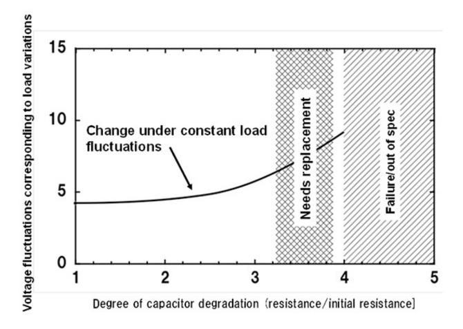
Figure 2: Relationship between the progression of electrolytic-capacitor degradation and amount of voltage fluctuations
