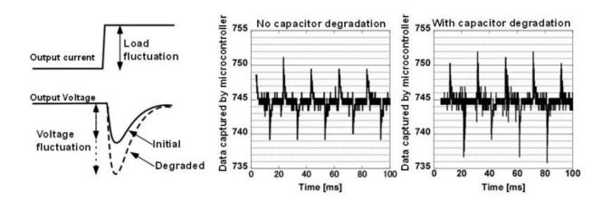
Figure 1: Output-voltage signal captured by microcontroller (fluctuation under load)
