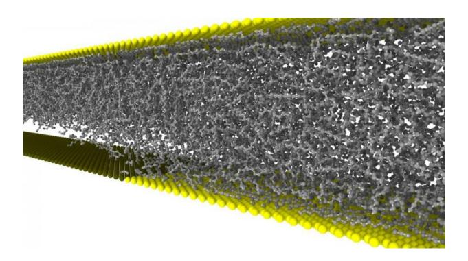
A cavitation bubble is formed in the lubricant between the oil-attracting (yellow) and the oil-repellent surface (black). When used as a buffer, it might reduce wear. Credit: KIT
