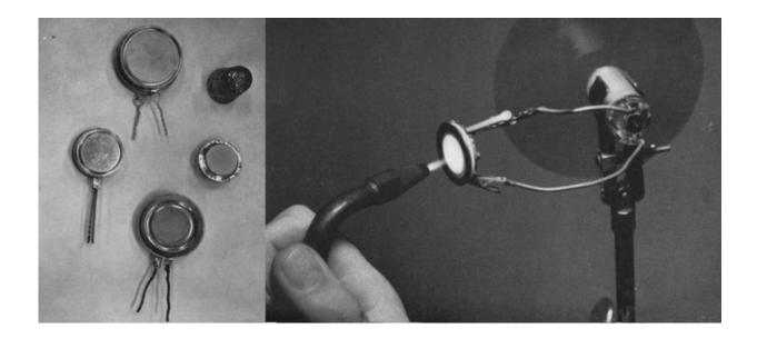
Hand-built research converters and thermionic demonstration device heated with a flame to produce power. Credit: GE Research, 1960s
