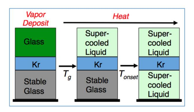
Inert gas permeation, a technique developed at PNNL, is used to investigate the formation of stable glasses.
