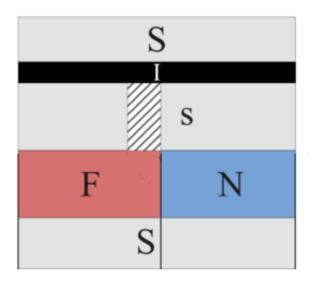
S – superconductor, I – insulating tunnel barrier, F – ferromagnet, N – normal metal, shaded area – potential barrier arising in the superconducting zone. Credit: Moscow Institute of Physics and Technology
