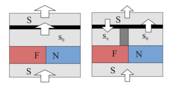
Superconducting currents when reading various states of the memory cell. The greater current the larger arrow. Credit: Moscow Institute of Physics and Technology
