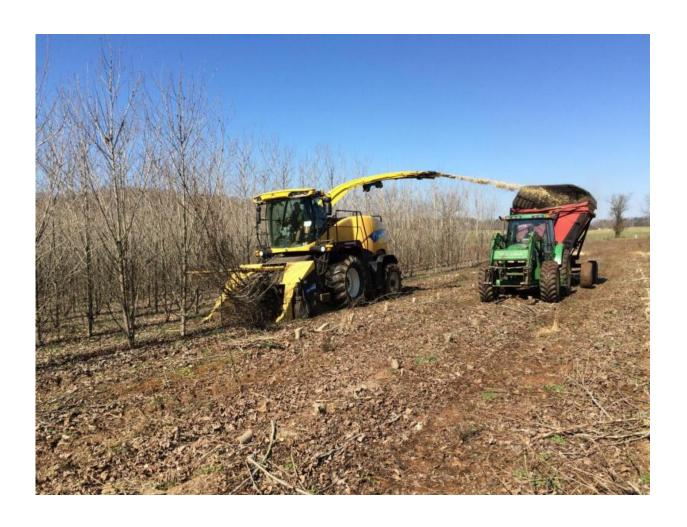
A self-propelled forage harvester with a specialized woody harvesting head harvests a 10-acre stand of hybrid poplars being studied to advance lignocellulosic biomass as part of a USDA-funded project coordinated by the University of Tennessee Center for Renewable Carbon. Credit: Genera Energy Inc.
