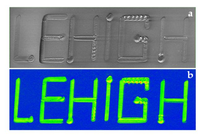
A scanning electron micrograph (a) and an image quality map (b) of that micrograph demonstrate the ability to fabricate patterned single-crystal architecture on a glass surface. In the lower image (b), the green color represents a single crystal embedded in the blue glass background. The width of lines in the two figures is about five micrometers. Credit: Dmytro Savytskii, Brian Knorr, Volkmar Dierolf & Himanshu Jain
