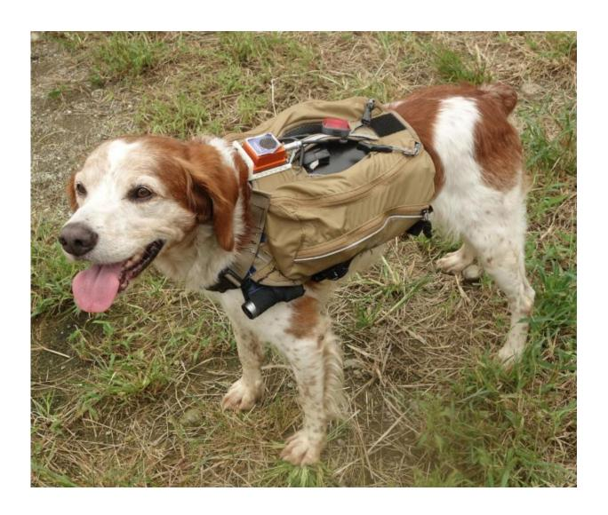
A recording vests for large size (25-30kg) and medium size (15-20kg) dogs. Device layout, its weight, and box shape were designed not to disturb SAR dog's activities. The vest was equipped with GPS, camera, and Inertial Measurement Unit (IMU). Handlers can confirm the camera image by a tablet PC. Credit: Tohoku University
