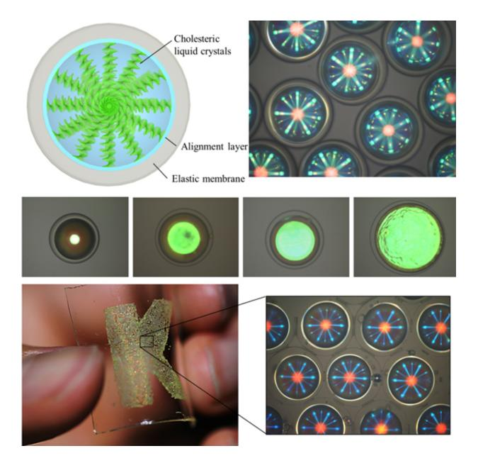
Composition of photonic microcapsules: cholesteric liquid crystal, alignment layer, and elastomer membrane from the core (top). Compression of single photonic microcapsule with high reconfigurability (middle). Assembly of photonic microcapsules to compose a photonic device (bottom). Credit: KAIST
