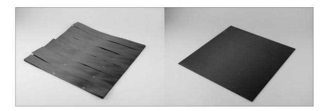
Carbon fibers and heated plastic combine under pressure to form a homogeneous CFRP plate. With infrared radiation in a vacuum, this occurs quickly and with a high degree of energy efficiency. Credit: Fraunhofer ICT
