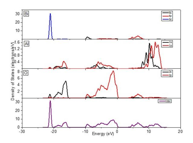
This is a diagram illustrating the variation of partial density of states for bismuth, aluminum and oxygen. Credit: MPLB
