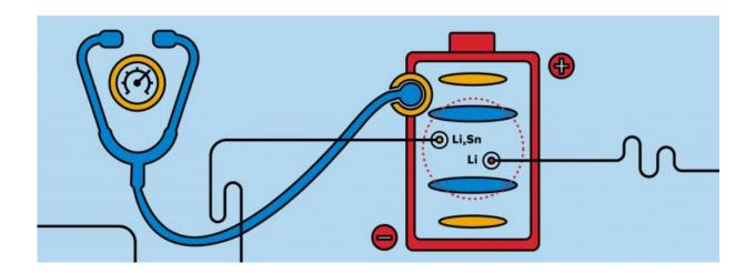
Reference electrodes provide insights into a battery cell's health. The image above depicts two reference electrodes within a battery cell. This configuration that allows researchers to evaluate a battery's anode and cathode separately at all stages of cycling and aging. Credit: Sana Sandler/Argonne National Laboratory
