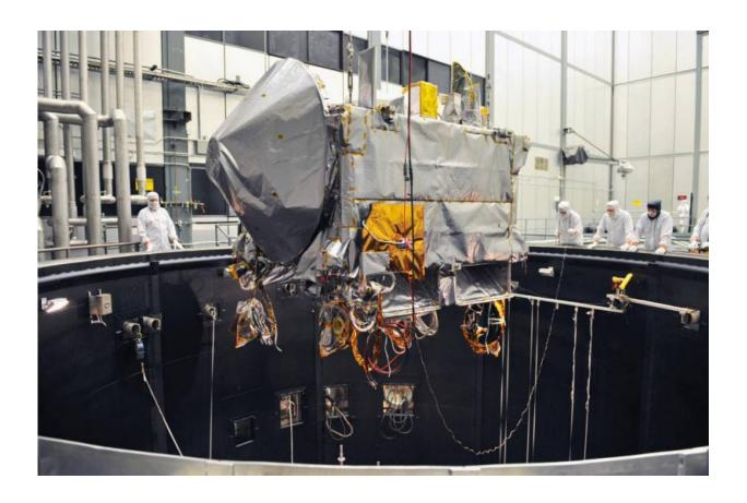
The OSIRIS-REx spacecraft being lifted into the thermal vacuum chamber at Lockheed Martin for environmental testing. Credit: Credits: Lockheed Martin
