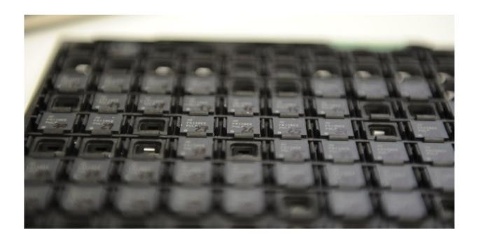
Series of PULP microprocessor chips on a tray. PULPino chips will be smaller, depending on technology and memory size as small as 1 x 1 millimeter. Credit: ETH Zurich / Frank K. Gurkaynak
