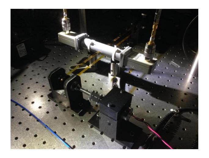
Measurements of electrical properties of a plastic tape (yellow), taken using a specially designed microwave cavity (the white cylinder at center) and accompanying electrical circuit, change quickly and consistently in response to changes in the tape's thickness. The setup is inspired by high-volume roll-to-roll
