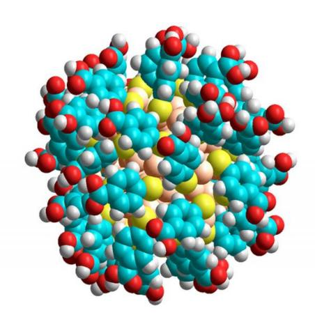
A gold nanoparticle: gold atoms are coloured pale orange, sulphur yellow, oxygen red, carbon cyan and hydrogen white.
