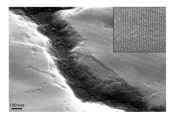
A scanning electron micrograph of a nanocrystal superlattice shows long-range ordering over large domains. Credit: Tisdale Lab
