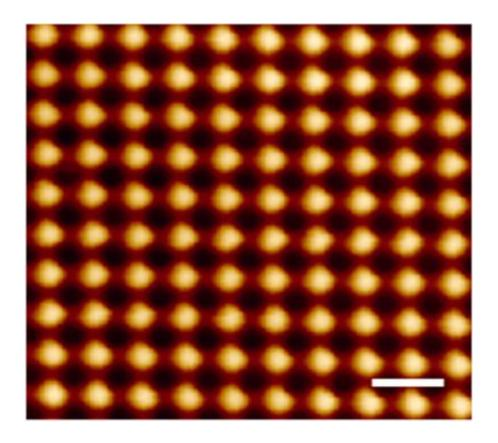
A 2D AFM image of BSTS nanocone arrays with d = 300 nm, h = 450 nm, and p = 600 nm. The scale bar is 1000 nm. Credit:
