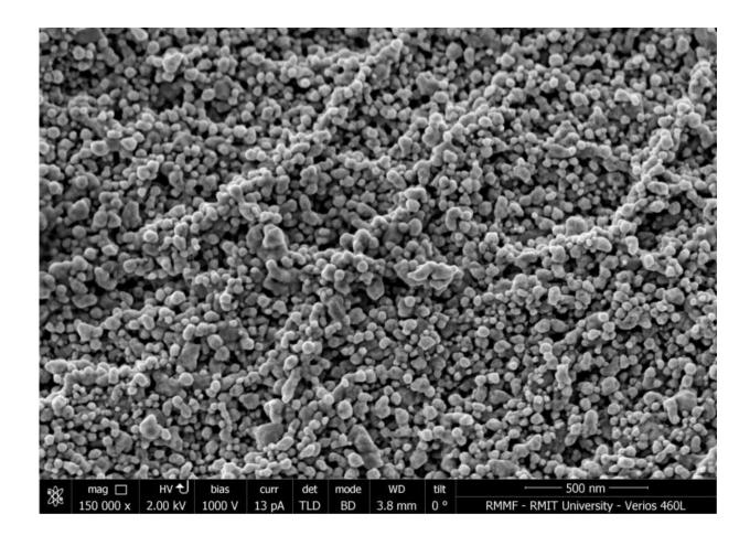
Close-up of the nanostructures grown on cotton textiles by RMIT University researchers. Image magnified 150,000 times. Credit: RMIT University
