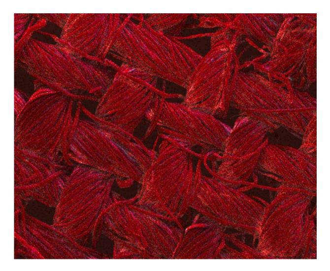
The red color indicates the presence of silver nanoparticles -- the total coverage on the image shows the nanostructures grown by the RMIT team are present throughout the textile. Image magnified 200 times. Credit: RMIT University
