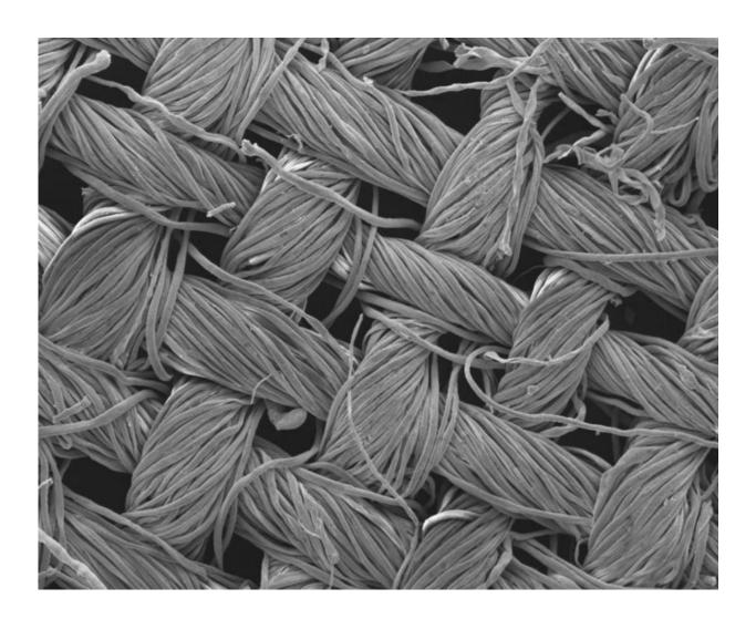
Cotton textile covered with nanostructures invisible to the naked eye. Image magnified 200 times. Credit: RMIT University
