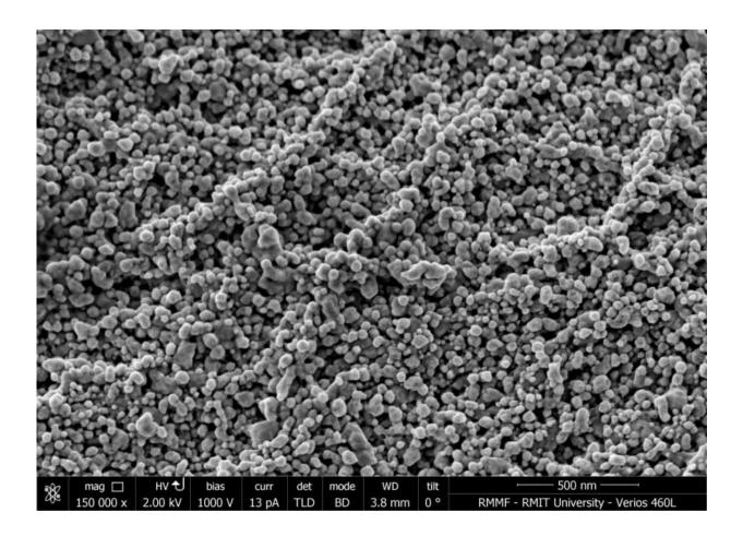
Close-up of the nanostructures grown on cotton textiles by RMIT University researchers. Image magnified 150,000 times. Credit: RMIT University
