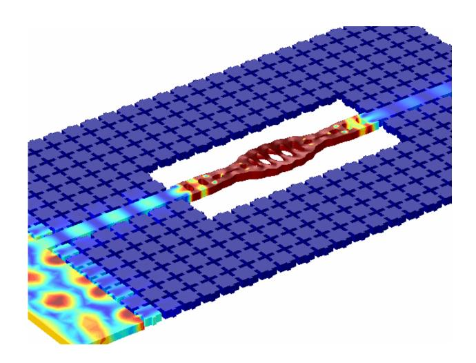
Acoustic waveguide channels phonons into the optomechanical cavity, enabling the group to manipulate the motion of the suspended nanoscale beam directly. Credit: K. Balram/K. Srinivasan/NIST
