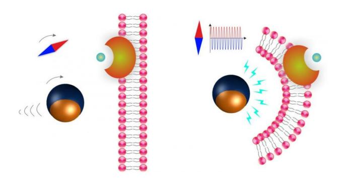
The Janus particles move by means of rotating magnetic fields (l.). If the magnetic field is altered, the microrobots generate an electric field (r.). A chemical compound (bluish green bullet) is released which than destroys defective cells. Credit: ETH Zurich / Salvador Pané
