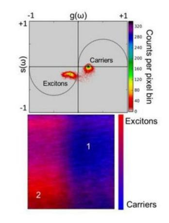
(Top) A phasor plot of the transient absorption data shows the presence of free charges and excitons; a false colored image shows their contributions at different spatial positions. Credit: ORNL
